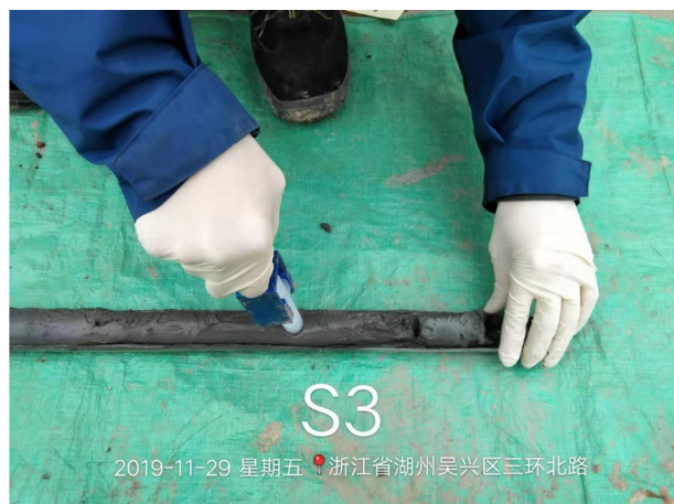
挥发性有机物非扰动土壤采样器装样
